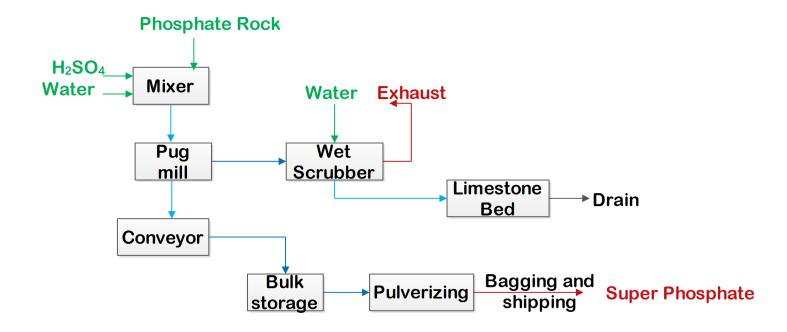
**Figure:** Manufacturing of Superphosphate
